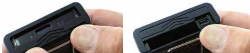
The battery door was designed to latch, providing extra security. To open, press at the lower right corner as shown. Slide the battery compartment door open, drop the battery in so that the connectors match and slide the battery door closed.
