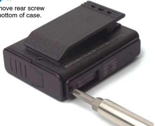
**Note:** Depending on date of manufacture, frequency adjustable models may or may not have a sliding door and bezel on this side. The screw is in the same location on both versions.
