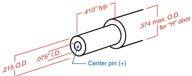
Mating Plug Dimensions and Polarity
