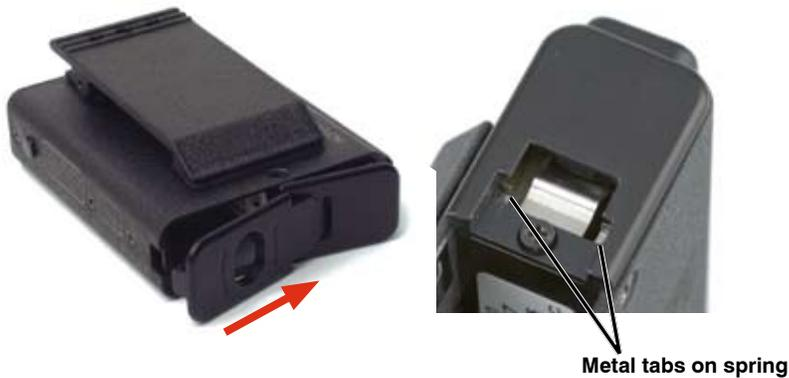
Re-align all parts before tightening screws. Tighten screw holding spring to the case bottom that was loosened in Step 2.
