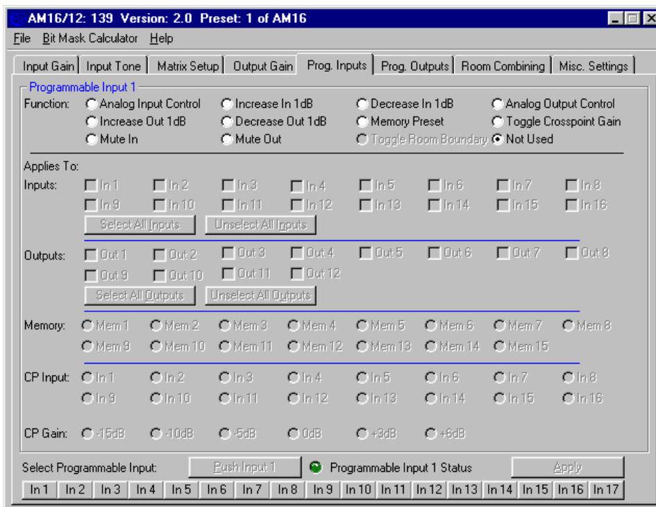
AM16/12 setup. Note that you should use the Select Programmable Input buttons to select the programmable input you'd like to configure before doing any configuration.
