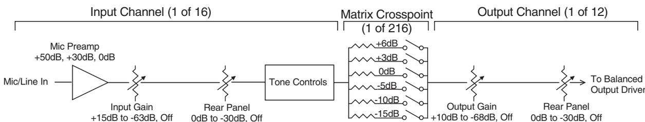
The diagram below represents the signal flow of one input to one output through one matrix crosspoint. Illustrated are all the gain control points in the signal path.
