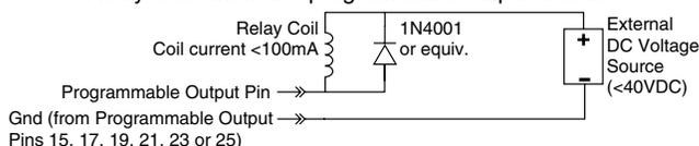
It is permissible to run LEDs from the +5VDC pins on the programmable input connector, as long as the total LED current for all LEDs on does not exceed 100mA. Similarly, 5V relay coils may also be run from the +5VDC pins on the programmable input connector, as long as the total coil current for all relays on does not exceed 100mA. Note that the diagram shows an external DC source powering the relay coil. This will be necessary if coil voltages above 5V are needed.
