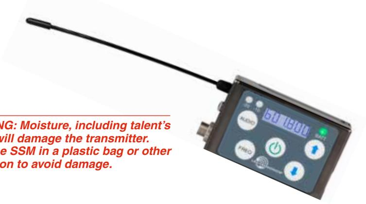
***WARNING: Moisture, including talent's sweat, will damage the transmitter. Wrap the SSM in a plastic bag or other protection to avoid damage.***
