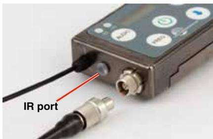
Place the transmitter close to the IR enabled receiver with the ports facing each other within a foot or two apart. Send the settings with the trigger on the receiver. If the settings are successfully transferred, a confirmation message will appear on the transmitter LCD.
