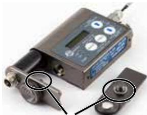
**Threads provide electrical contact**
