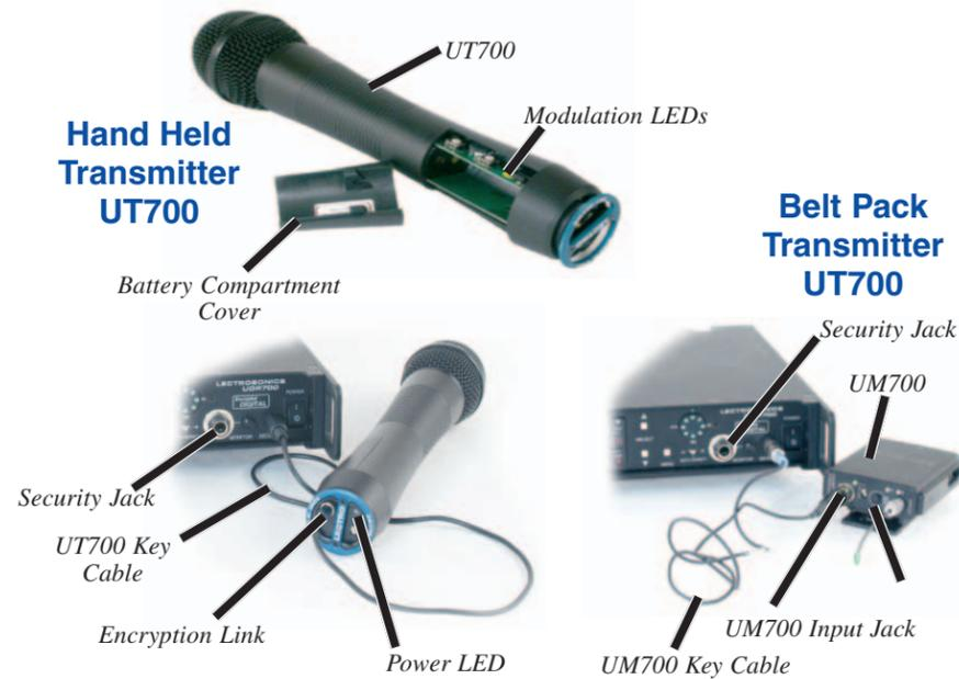
10) **Transfer Encryption Key** - Turn on the transmitter, verify battery condition, and then press the SELECT Up on the UDR700 to transfer the encryption key to the transmitter. The Power LED on the UT700 and the two Modulation LEDs on the UM700 blink to confirm receipt of the new key.
