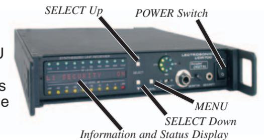
8) **Generate Encryption Key -** Press MENU to enter the Key Generation Menu. "MAKE NEW KEY? ^" will be displayed in the Information and Status Display.
