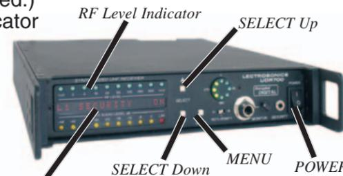
If a clear channel is not available using one of the factory preset frequencies, press and hold the MENU button, then press the SELECT Up or Down button to tune across the entire 25.5 MHz frequency block (in 100 kHz steps) to locate one.
