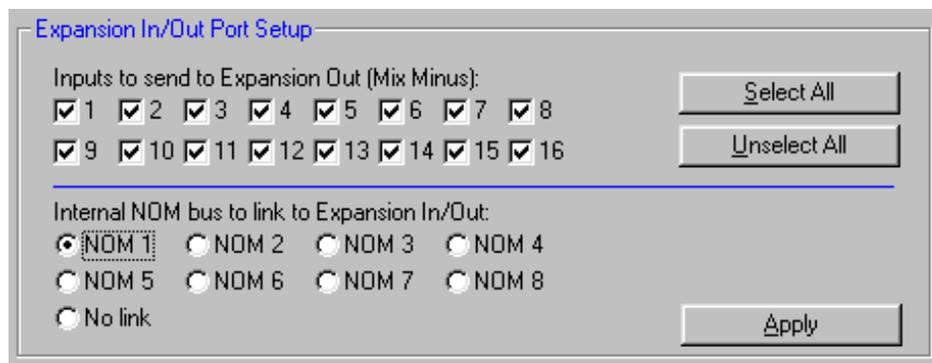
Notice that all the Input boxes are checked, which will send the signals from all inputs to the Expansion In Mix Minus pin. In addition, since all the inputs are associated with AM16 NOM bus 1, the Expansion port should be also. The Apply button must be clicked before any of the changes made in the Expansion In/Out Port Setup frame will be active.
