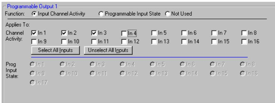
Note that on the Misc Settings tab, the input qualification time and output hold time may be set to optimize the time response of channel activity for various applications. The screen below shows programmable output 1 responding to activity on any of input channels 1, 2, or 3.
