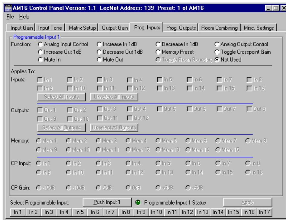
the Select Programmable Input buttons to select the programmable input you'd like to configure before doing any configuration.
