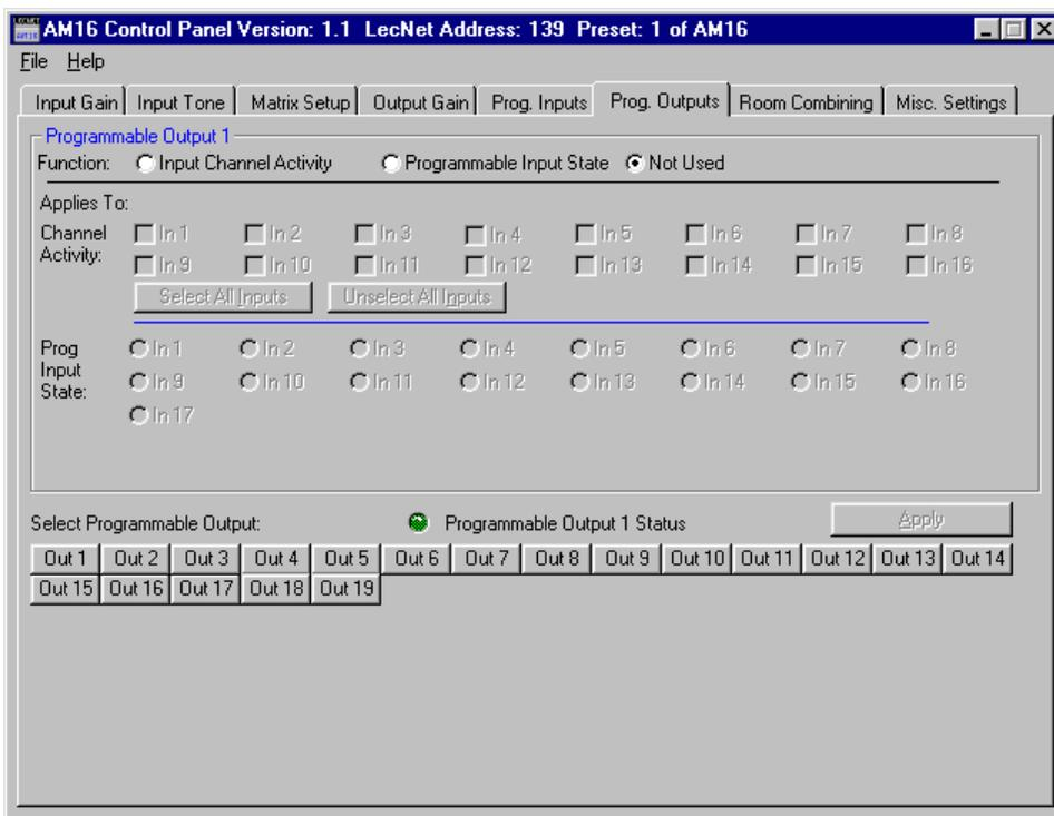
*Hint:* If the function (or any associated channels or programmable inputs) of a programmable output is changed on the control panel, the **Apply** button will be enabled. The **Apply** button is located in the lower right hand corner of the Programmable Output tab. The **Apply** button must be clicked before any changes are actually applied to the active AM16 setup.
