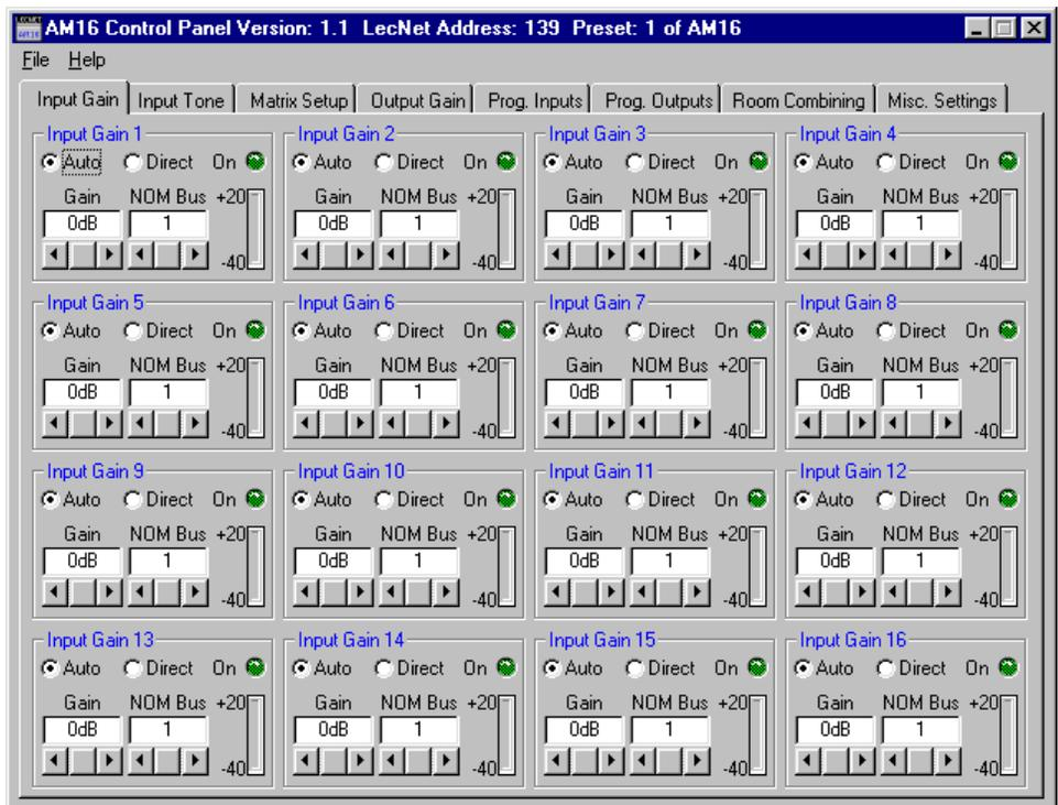
**Short Cuts:** A left mouse click on the gain box will set the input gain to 0dB, while a right mouse click will set the input gain to Off.
