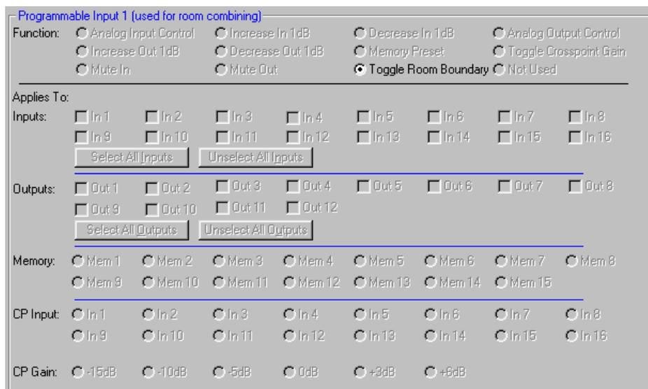
**Mute In / Mute Out** - Allows one or more inputs (Mute In) or outputs (Mute Out) to be temporarily muted. The first momentary contact closure on the programmable input pin will mute the specified input(s) or output(s), and the next momentary contact closure will unmute them. The screen to the right shows that programmable input 1 is set to mute inputs 1, 2, 3, and 4.
