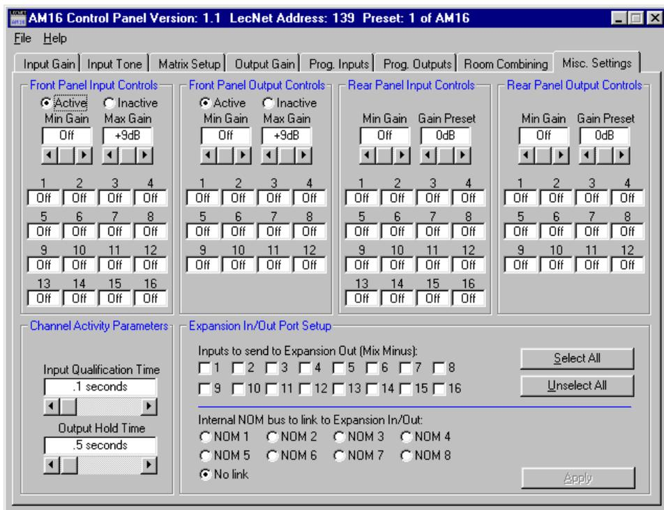
*Short Cuts:* A left mouse click on the Min Gain box will set the minimum gain to Off (i.e. no limit on the minimum gain), while a right mouse click will set the minimum gain to -1dB. A left mouse click on the Max Gain box will set the maximum gain to +9dB, while a right mouse click will set the maximum gain to +1dB.
