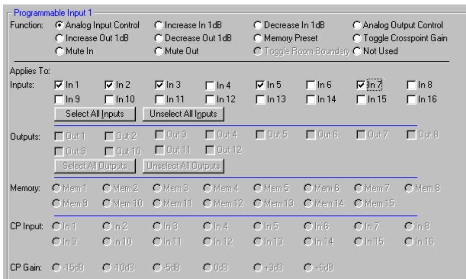
contacts to the programmable input pin and ground. The inputs will be muted when the contacts are closed. The screen shown to the right indicates that the function of programmable input 1 is analog input control of inputs 1, 2, 3, 5, and 7. Notice how multiple inputs may be controlled by a single programmable input.
