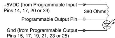
Relay is on when the programmable output is active
