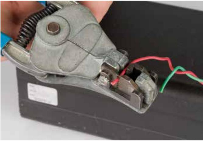
**3.** Strip the insulation back approximately 1/8 inch and twist the bare strands for easier insertion into terminals as shown in step 4.
