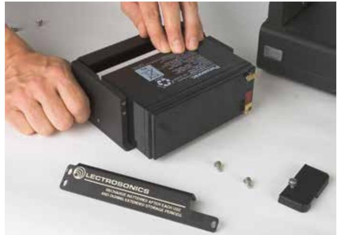
**7.** Push the battery out of the mounting assembly from the side opposite the retaining bracket.
