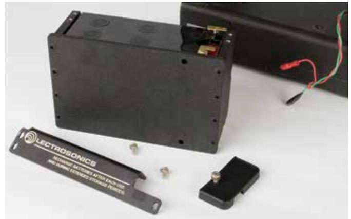
**6.** Remove the terminal cover and the retaining bracket from the new battery assembly.
