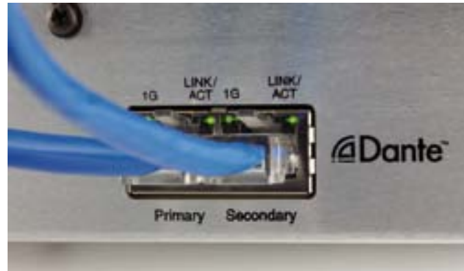
The built-in Ethernet switch allows operation with either port in the Switched mode with a single network, and as primary and secondary ports in the Redundant mode with two networks.
