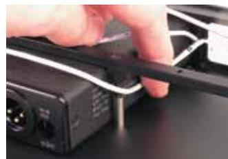
*With each receiver, route the "B" antenna cable under the bar and place it in the gap next to the screw.*
