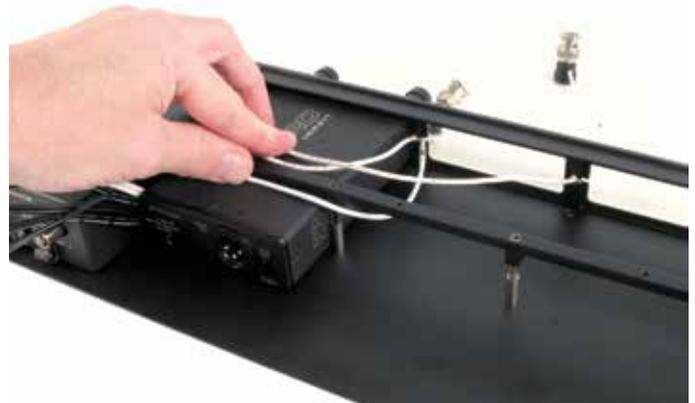
5. Secure the receivers into the frame by tightening the five counter-sunk phillips head screws in the rectangular metal rod. **Don't overtighten!**
