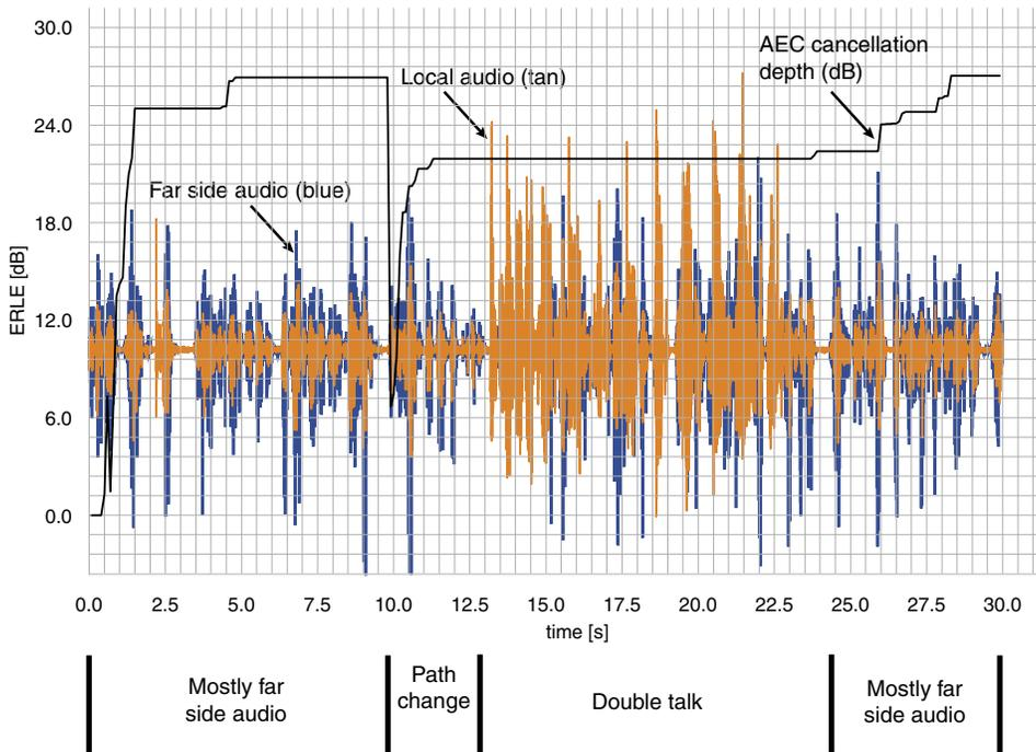
When a local sound system is being used to amplify only far side audio, the AEC can quickly identify and cancel the far side audio that enters the local microphones.
