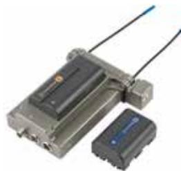
The receiver can be powered with an optional battery "sled" adapter that accepts standard "L" and "M" style rechargeable batteries. The adapter includes an integrated SREXT plate for the rear panel audio outputs. Typical runtime with a 7.2 V, 2200 mA "L" style battery is approx. 11 hours.
