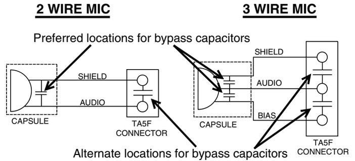
Install the capacitors as follows: Use 330 pF capacitors. Capacitors are available from Lectrosonics. Please specify the part number for the desired lead style.
