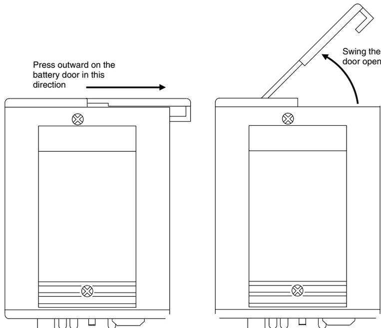
Insert the battery correctly and close the cover by pressing the door closed and across, reversing the opening procedure illustrated above. If the battery is inserted incorrectly, the door will not close. Do not force the door closed.
